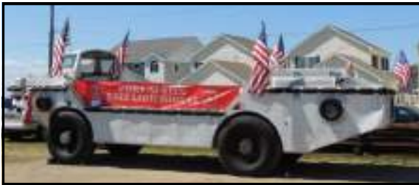
LARC-V (Lighter, Amphibious Resupply, Cargo, 5 ton), is an aluminum-hulled amphibious cargo vehicle capable of transporting 5 tons or 28 passengers. It was developed in the United States during the 1950s, and is used in a variety of auxiliary roles to this day.
